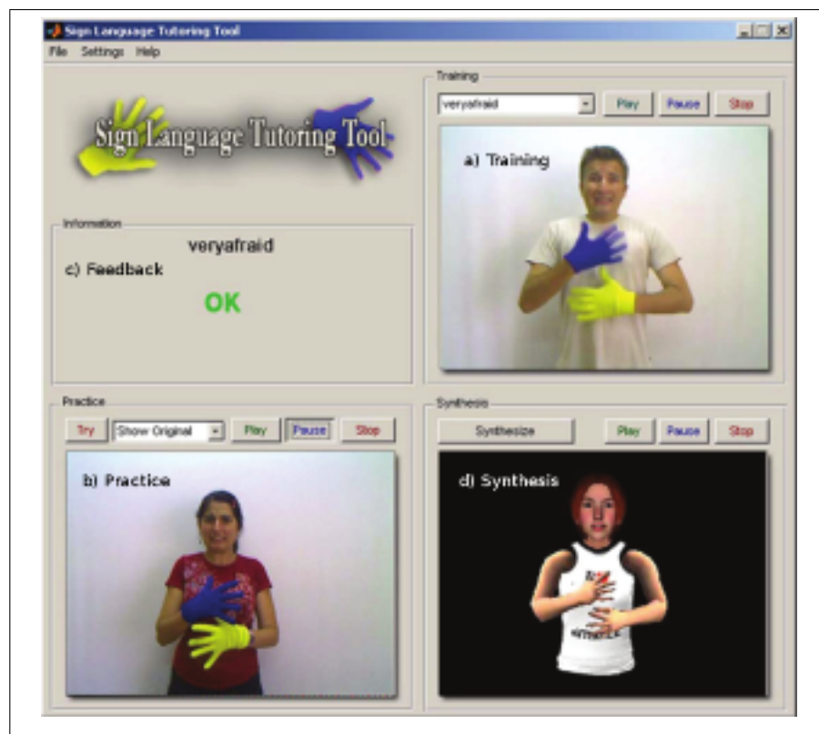
Figure 1.1. Sign Tutor GUI: a) Human learners can view videos recorded in the database for training. b) Performance of the human learner is recorded through a webcam, and then displayed. c) The system analyses the performance and provides feedback verbally as OK or WRONG . d) System can also provide an animated feedback.
