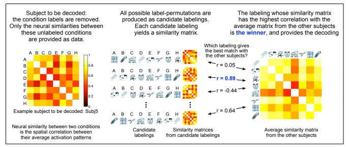
**Figure 1.** Our novel method of across-subject neural decoding: DEMOSS. The data entered into the model for each subject consists only of the values in their  $8 \times 8$  similarity matrix, constituting  $8 \times (8 - 1)/2 = 28$  unique numbers. Only one permutation-matching computation is performed per subject, so there are no multiple comparisons. The illustrated similarity matrices are the actual data for the example subject shown.
